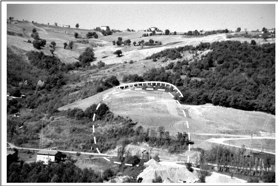
Fig. 1 – Panoramic view of the slope where the Ca’ Bonettini landslide took place. Broken lines represent the landslide’s crown and body (courtesy of D. Castaldini)
