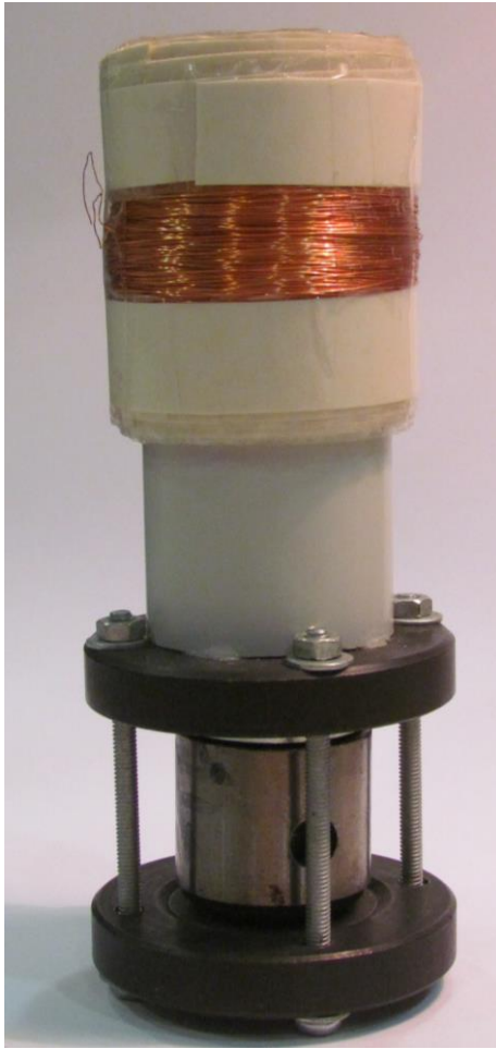
Figure 9 Harvester prototype on the vibrating table
