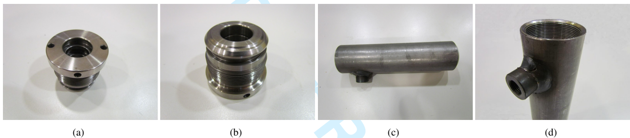
Figure 2. Commercial components. Cylinder head for a 20 mm diameter rod (a), (b). Hydraulic cylinder (c) and welded boss for pressurization system (d).
