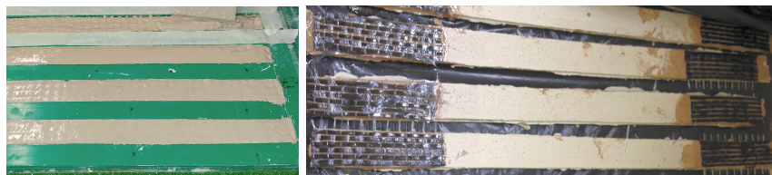
Figure 3: Two stages in specimen manufacturing: specimens cure in the modular formwork (left) and, after stripping, they are provided with end tabs (right).
