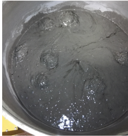
Figure 4: Phenomenon of fiber balling occurred in HF85 series
