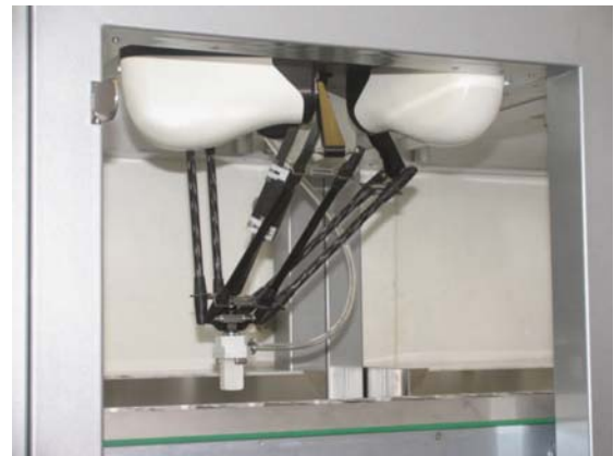
Figure 1. Robot with the Delta structure used in the proposed application: Codian D4-500 [5].
