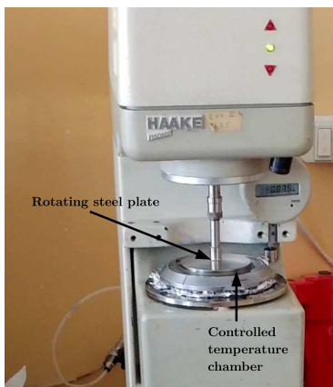
Figure 4: Rheometer test set-up
