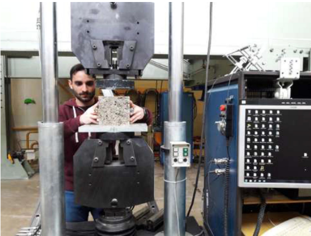
Fig. 10. Compression test setup.
