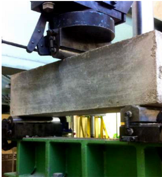
Fig. 16. Bending test setup.
