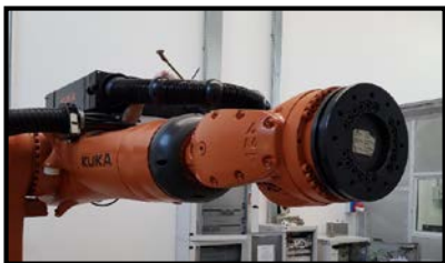
Fig. 15a. Load Type 1: no additional load applied on the IR end effector.
