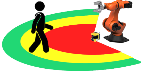
Figure 2: Safety zones for human-robot collaboration with speed and separation monitoring technology (Courtesy of ABB Robotics).
