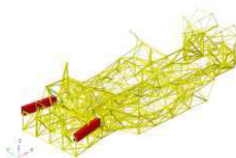
Figure 10. Second model variant results (maximum admissible stress 50 MPa).
