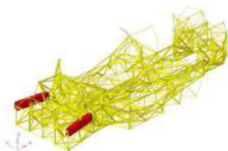
Figure 9. Second model variant results (maximum admissible stress 40 MPa).
