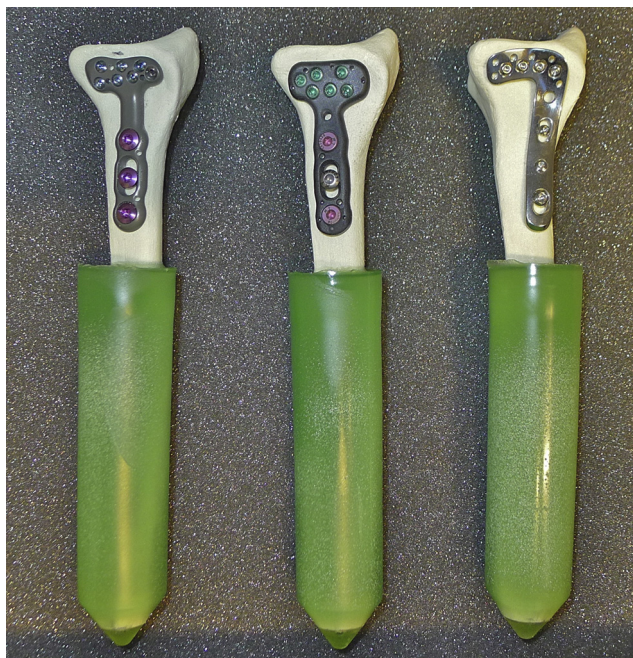
Fig. 1. Plates tested. From left to right: titanium DVR (Hand Innovations, Miami, FL); CFR-PEEK DiPHOS-RM (Lima Corporate, San Daniele Del Friuli, Udine, Italy); stainless steel volar lateral column (Zimmer, Warsaw, IN).
