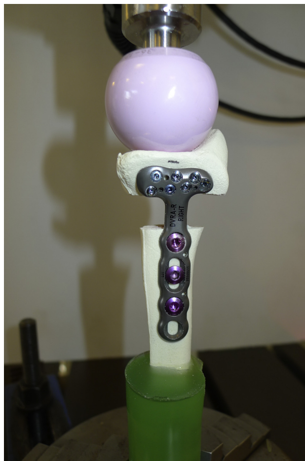
Fig. 2. Axial loading test performed by advancing a ceramic sphere centered over the lunate fossa at a constant rate of displacement of 5 mm/min.
