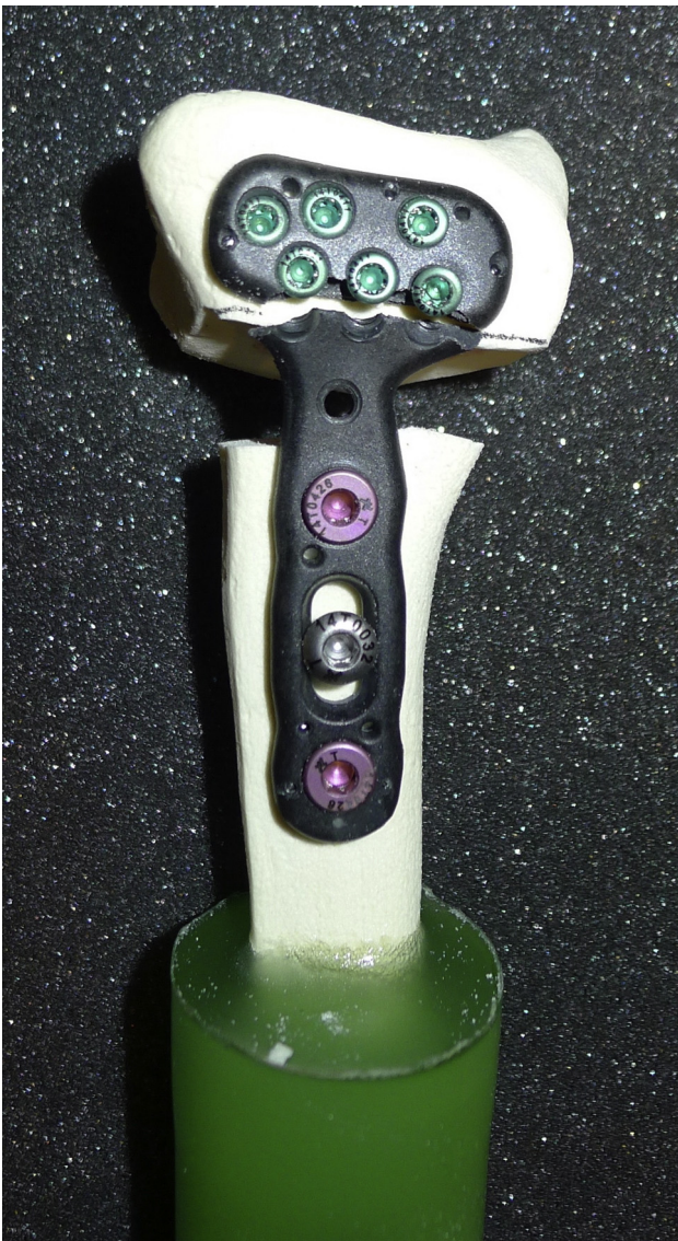
Fig. 6. CFR-PEEK plate breakage line at the proximal row holes on the head portion of the plate during both pre and post-fatigue axial loading tests.
