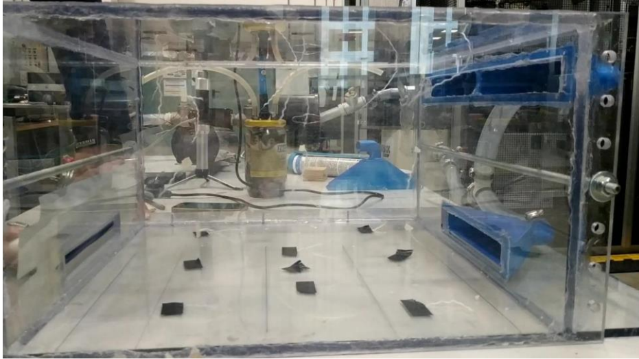
Figure 40: configuration of the flags inside the chamber
