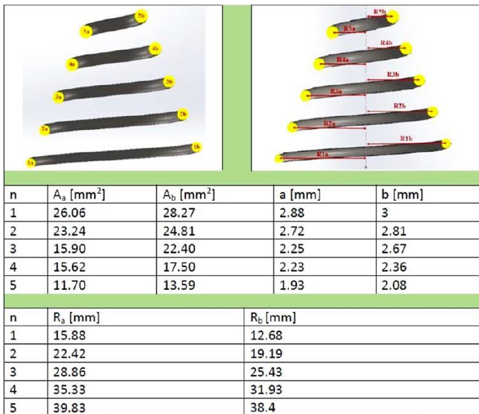
Figure 82: geometric characteristics of the printed spring
