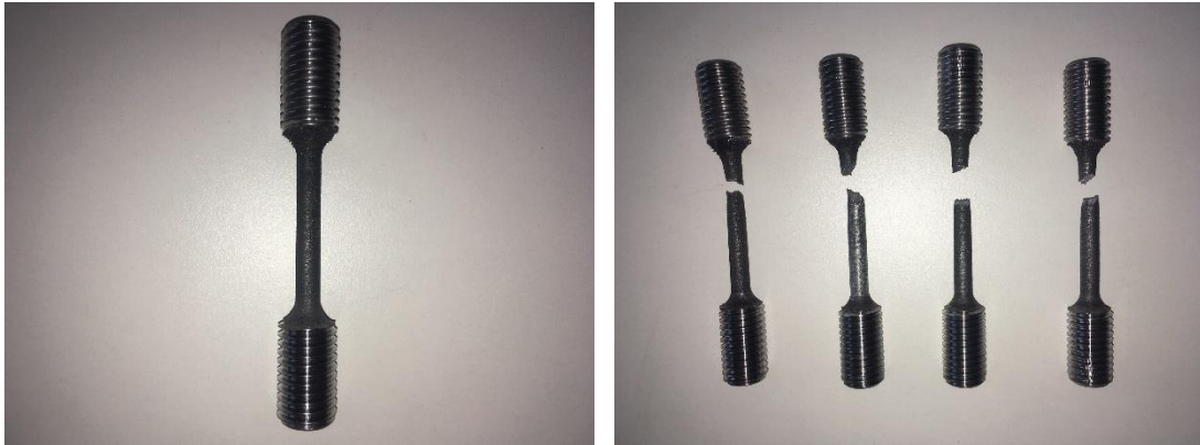
Figure 110: picture of the sample. A) sample before the test - B) samples after tensile tes
