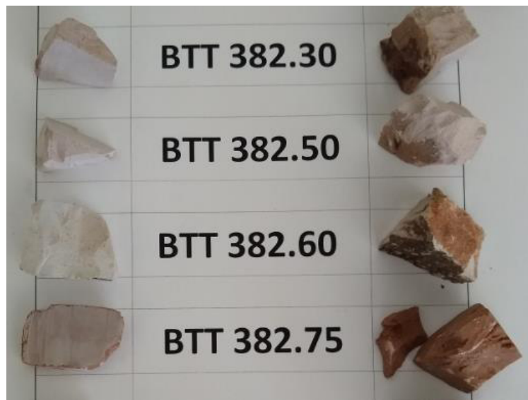
Figure 3.19: Samples of the Bottaccione sequence, (Gubbio Italy). On the right, the witnesses preserved after the cut; on the left, the chips, cleaned from the superficial alteration, which were then powdered.
