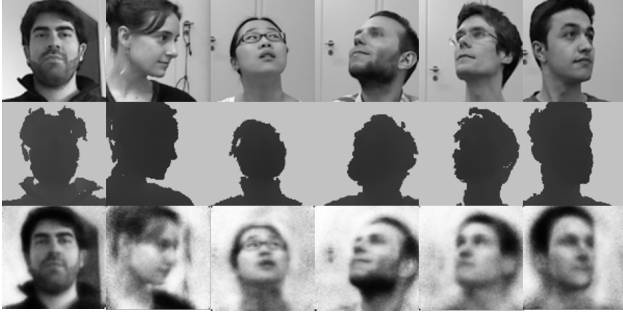
Figure 2. Examples of gray-level face images (bottom) reconstructed from the depth maps (middle). The corresponding ground truth is also shown (top). The first four subjects have been included in the training set, while the last two are completely new.
