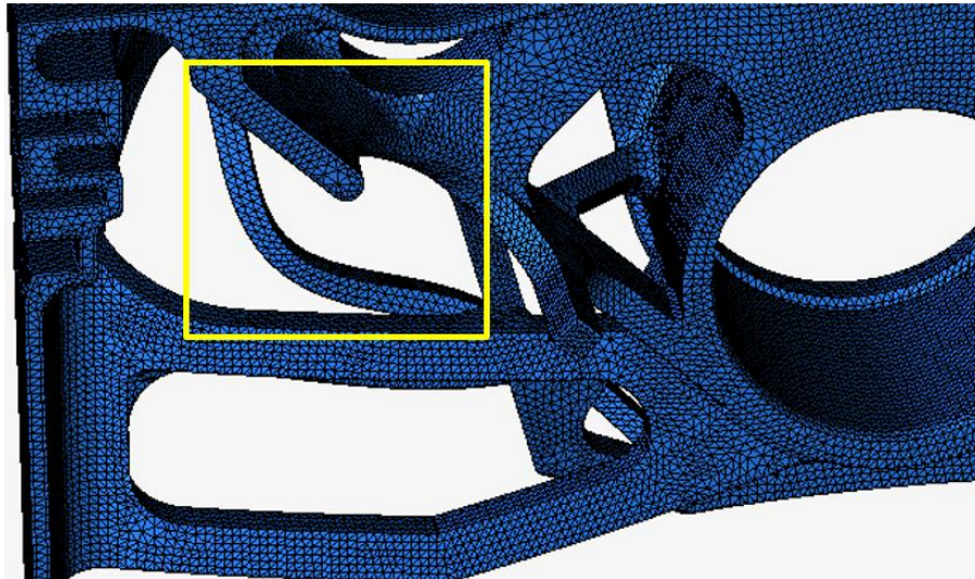
Figure 8.22. TDCI, buckling collapse.
