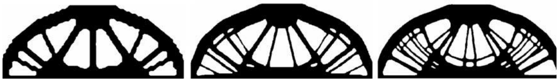
Figure 5.4. A different mesh density can lead to a different topological distribution [43].
