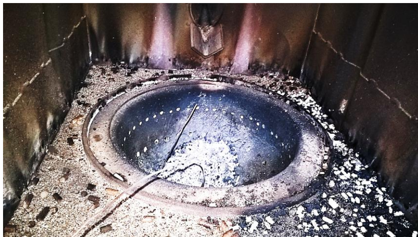
Figure 4. Ash in the combustion chamber after the P 100 test
