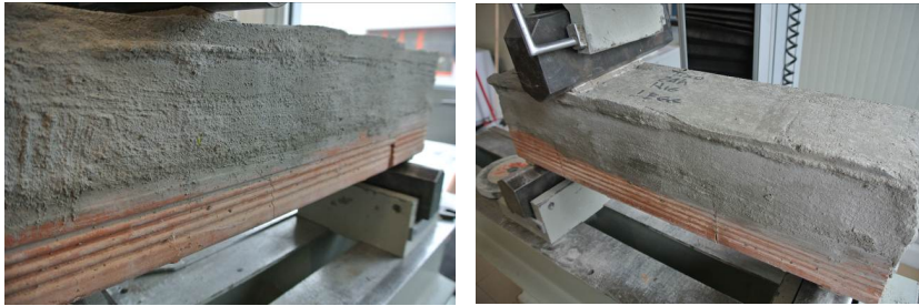
Figure 1: Ceiling beams for flooring stiffened by a casted repairing mortar layer.
