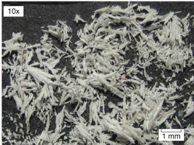
Figure 7: Wear debris of polyamide 66 after 20 km of sliding against dry steel counter-surface, at 90 N [12].
