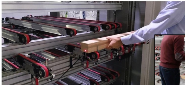
(A) Fixed loader (uncomfortable positions for loading)
