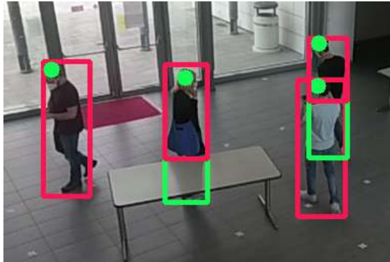
Fig. 13. Examples of CenterNet bounding boxes (pink), refined bounding boxes and head localization (green).
