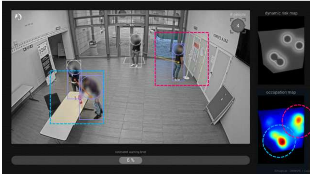
Fig. 12. GUI of our system. In the main frame, anonymized bounding boxes are superimposed to the image. Colored links encode people reciprocal distance. On the right, two maps show the bird-eye view of the area. The estimated risk level of the scene resides at the bottom of the interface.
