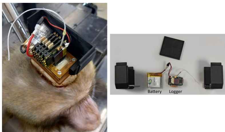
Figure 7. The recording chamber divided in its components. On the left, the recording chamber open; on the right, the battery connected with the recording system (RatLog-128 from Deuteron technologies) between different parts of the headcap.
