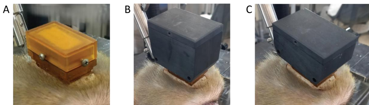
Figure 6. Implant system design. A) Home-cage configuration; B) Primate-chair configuration; and C) Freely-moving animal configuration.
