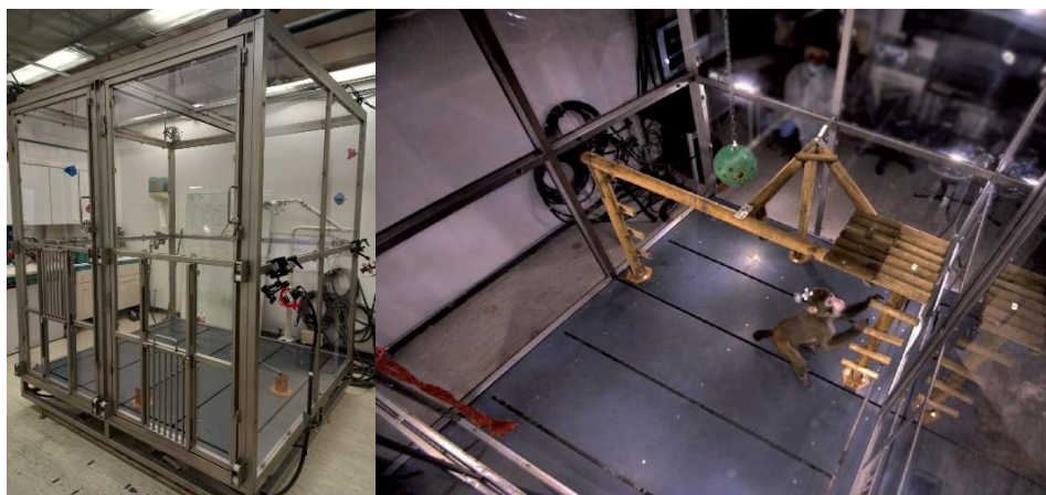
Figure 8. The NeuroEtoRoom (NER), a large plexiglas enclosure where the sessions are recorded. On the left, a view from the outside, when the enclosure is empty; on the right, a view from the inside, while the monkey is freely moving around the enriched cage.
