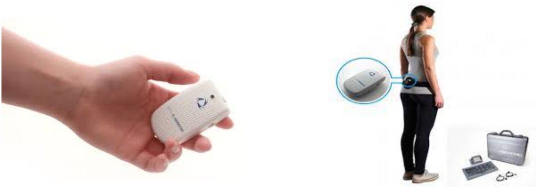
Fig. 2 G-Walk inertial device used in this thesis and its positioning
