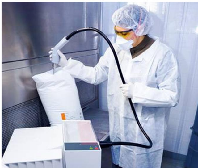
Figure 2.3.4. Example of use of FOP for raw materials quality control.
