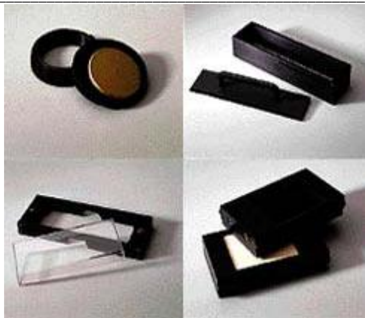
Figure 2.3.2. Different sample cells with quartz window for NIR diffuse reflectance spectroscopy.
