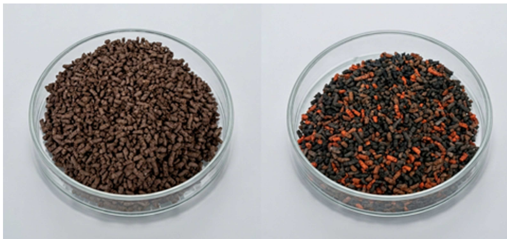
FIGURE 1 | Photos, respectively, of raw ABVF pellets (left) and fired ABVF pellets (right).
