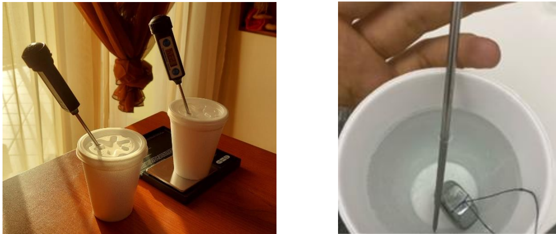
Figure 4. Polystyrene cups, digital scale and thermometers employed in a measurement of latent heat of ice. Only one cup and one thermometer are needed for this experiment. By also using a steel nut used in the Hooke's Law experiment, the specific heat of steel can be measured.
