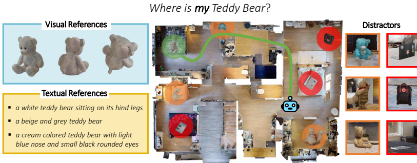
Figure 5.1: We introduce the PIN task, where the agent is asked to navigate toward a personalized object instance using multimodal references and distinguish it from distractors ( i.e. , other objects of the same category as the target or of other categories). The target object, same category distractors, and other distractors are circled, respectively, in green, orange, and red. The total number of available objects in the dataset is 338, corresponding to different instances of 18 object categories.
