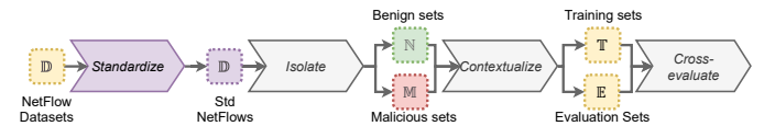
Fig. 3: Overview of XeNIDS. The input \mathbb{D} is a set of labelled NetFlow datasets of n distinct networks. The output results should be further analyzed.
