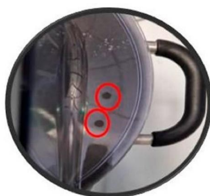
Figure 2. Details of the upper closure of the planetary mixer showing the perforated section used for gas sampling during VOC monitoring.
