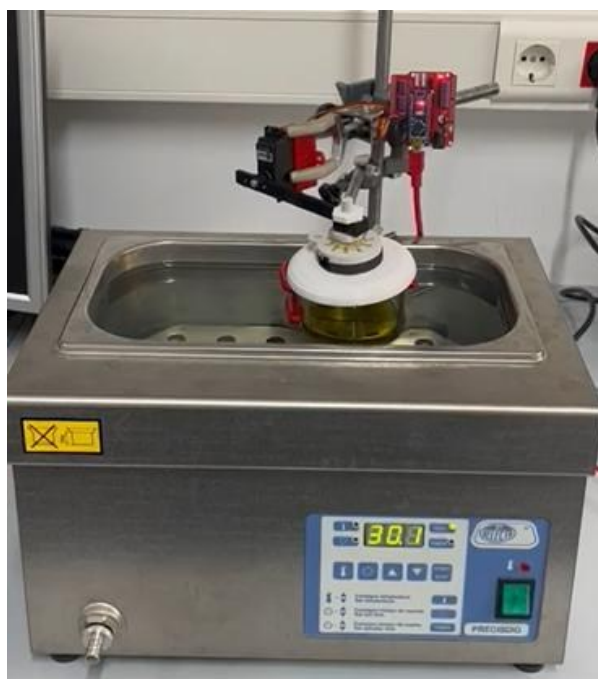
Figure 1. Analysis of oil samples using an electronic nose.
