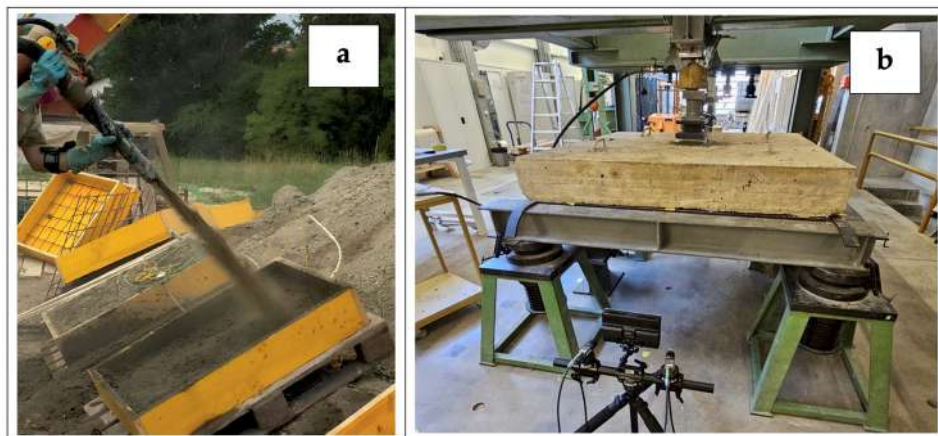
77 78 Fig. 2. (a) Shot-Earth projection leaned 45° over the horizontal direction (from [9]), (b) Test of a Shot- 79 Earth slab
