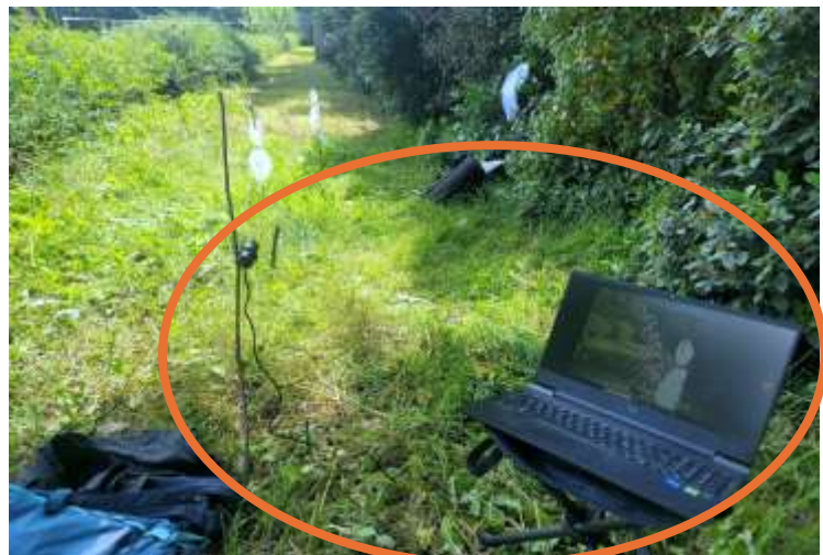
Figure 4. 4: micro Dinolite camera used for recording the insects visiting H. adriaticum plants in Parco S. Lazzaro, linked to the laptop to save and identify the insects later.
