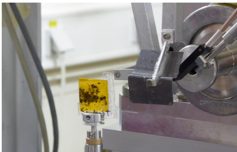
Fig. 2.4.12. Standard powder of Si NIST embedded between glass supported kapton sheets.
