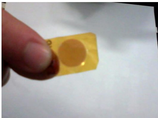
Fig. 2.4.10. Pellet of erionite sample sealed between kapton foils.
