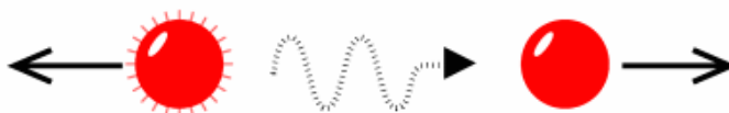
Fig.2.3.4. Recoil of free nuclei in emission or absorption of a gamma-ray (from www.rsc.org ).
