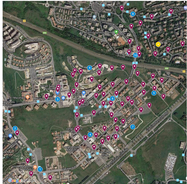
FIGURE 5. Torino-MezzoCammino terrain view including: Measurement points (bordeaux pins), center of the areas (blue pins) and macro cell (MC) position (yellow pin).
